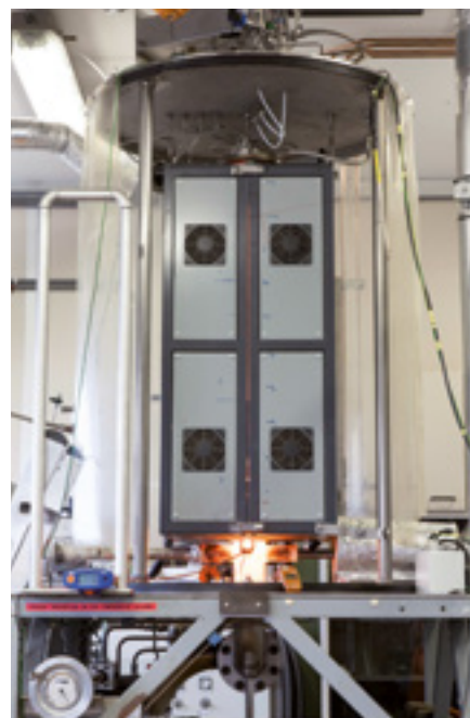
Lab-scale Combustion and gasification Simulator (LCS) for Pulverised Fuel testing.
