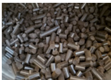
TORWASH® pellets from sewage sludge
